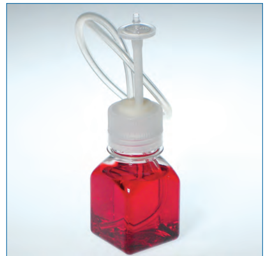
Single 60mL sampling bottle showing Bio-Simplex™ Closure Assembly with an EZ Top® container closure.
